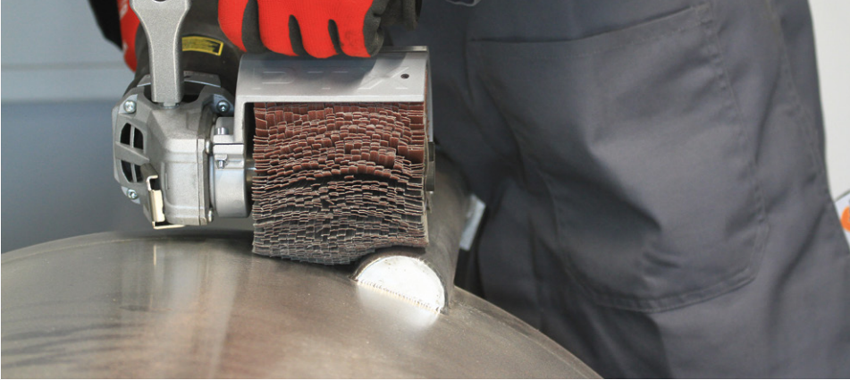
The scrubby wheel adapts perfectly to the fillet weld.
